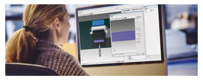
Master BendCam is the modern and automated CAD-CAM for all Prima Power panel benders and uses advanced 3D simulation for controlling the feasibility of parts before starting the real manufacturing process. It uses interactive graphic techniques to simulate the bending process in a realistic way, generating optimised and safe programs.
